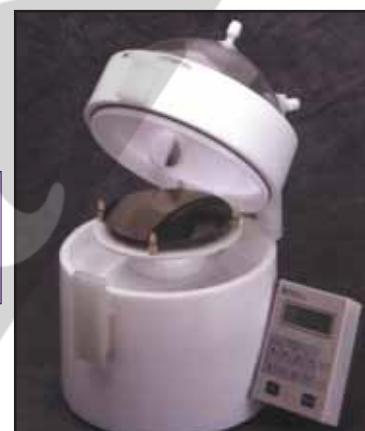
Figure 5. Spin-coater for deposition on wafers.
