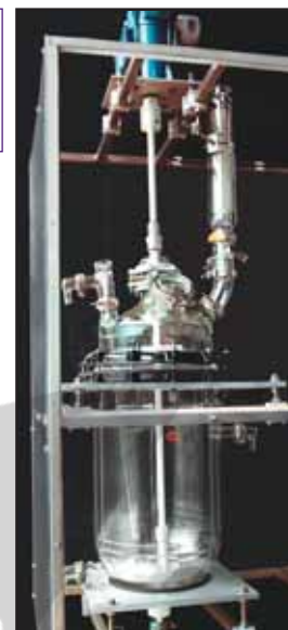
Fig. 1 Reactor for slurry treatment of powders. Separate filtration and drying steps are required.
